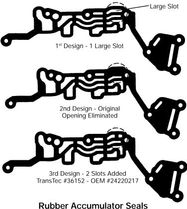
The lathe (square) cut accumulator seals in this kit are TransTec's aftermarket design seals. The dimensions are slightly different, and the material is more abrasion-resistant than the OEM seals. The design of these seals was improved because of occasional wear problems with the OEM seals. The transmissions most affected are the 4T60/E and AXOD, due in part to the design of these accumulators.
