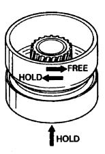
Must rotate counterclockwise and hold clockwise
